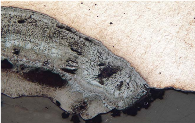
Fig. 4. \text{PbSO}_4 corrosion product on negative strap. Magnification 70 \times .
