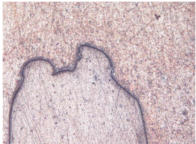
Fig. 10. Weld area of TASC strap showing no corrosion. Magnification 35×.
