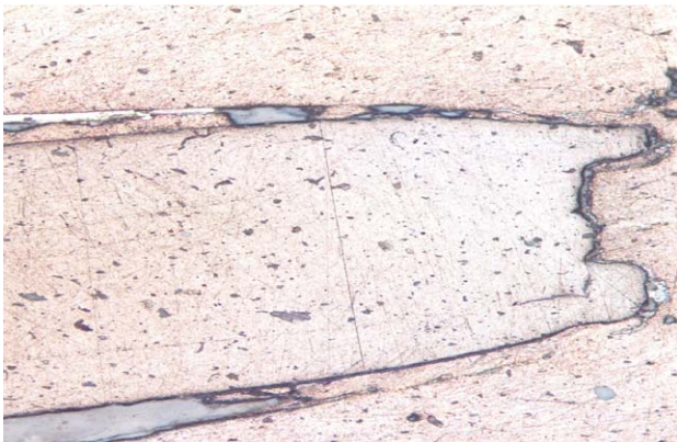
Fig. 5. Growth of corrosion product on both sides of plastic cell wall. Magnification 35 \times .
